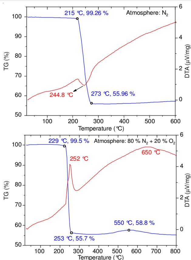
Fig. 3. TG and DTA curves of  $[\text{Pt}(\text{NH}_3)_4](\text{C}_2\text{O}_4)$  in inert and in oxidative atmosphere
