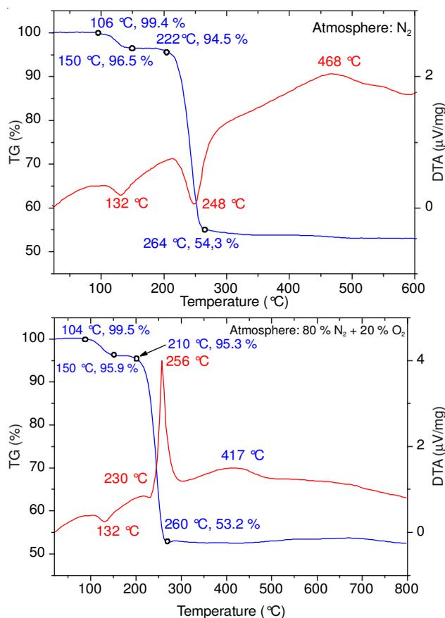
Fig. 4. TG and DTA curves of  $[\text{Pt}(\text{NH}_3)_4](\text{OOCCH}_2\text{COO})$  in inert and in oxidative atmosphere
