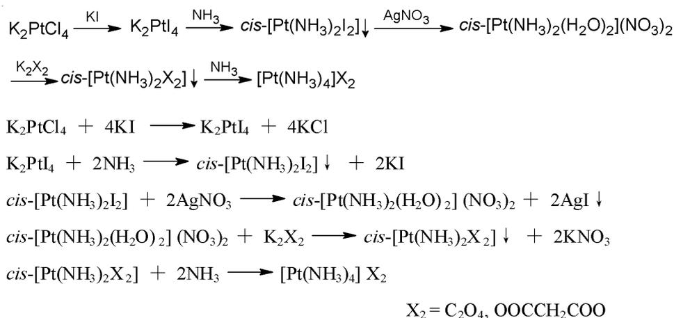
Fig. 1. Synthetic scheme and reactions of [Pt(NH<sub>3</sub>)<sub>4</sub>](C<sub>2</sub>O<sub>4</sub>) and [Pt(NH<sub>3</sub>)<sub>4</sub>](OOCCH<sub>2</sub>COO)
