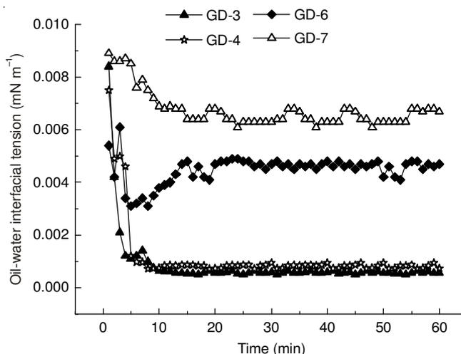
Fig. 8. Dynamic interfacial tension of GD oil block
