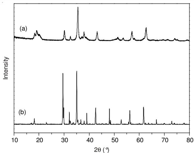
Fig. 2. XRD of cross-link magnetic chitosan nanoparticles (a) and  $\text{Co}_{0.5}\text{Mn}_{0.5}\text{Fe}_2\text{O}_4$  particles (b)
