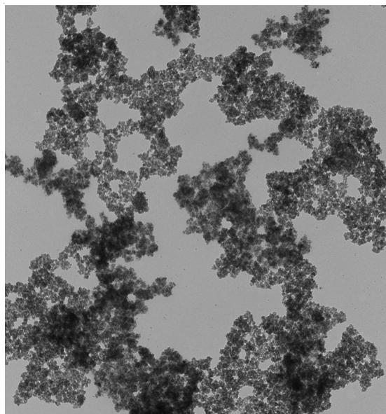
Fig. 4. TEM micrographs for the  $\text{Co}_{0.5}\text{Mn}_{0.5}\text{Fe}_2\text{O}_4$ -chitosan nanoparticles
