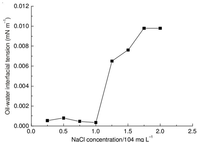
Fig. 10. Effect of sodium ions to interfacial tension
