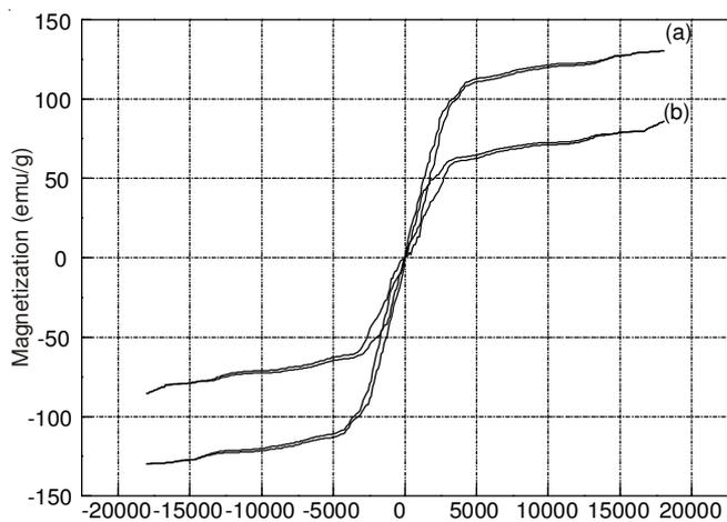
Fig. 7. Field dependence of magnetization for the  $\text{Co}_{0.5}\text{Mn}_{0.5}\text{Fe}_2\text{O}_4$ -chitosan nanoparticles (b) and  $\text{Co}_{0.5}\text{Mn}_{0.5}\text{Fe}_2\text{O}_4$  nanoparticles (a)
