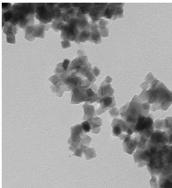
Fig. 3. TEM micrographs for the  $\text{Co}_{0.5}\text{Mn}_{0.5}\text{Fe}_2\text{O}_4$  particles
