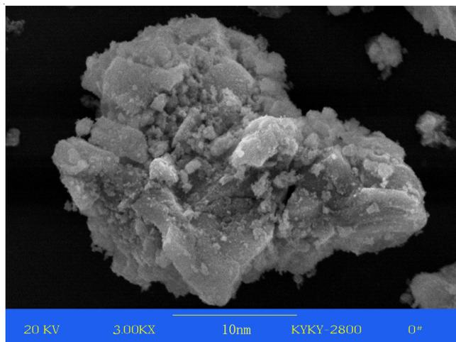
Fig. 5. SEM micrographs for the  $\text{Co}_{0.5}\text{Mn}_{0.5}\text{Fe}_2\text{O}_4$  particles
