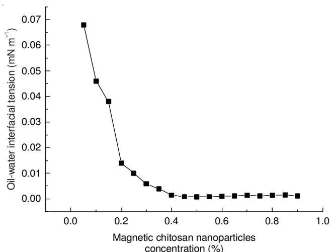
Fig. 9. Effects of  $\text{Co}_{0.5}\text{Mn}_{0.5}\text{Fe}_2\text{O}_4$ -chitosan nanoparticles contents on the interfacial tension
