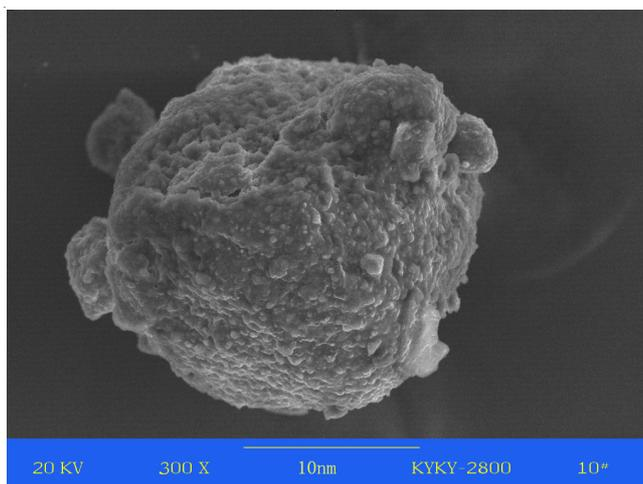
Fig. 6. SEM micrographs for the  $\text{Co}_{0.5}\text{Mn}_{0.5}\text{Fe}_2\text{O}_4$ -chitosan nanoparticles
