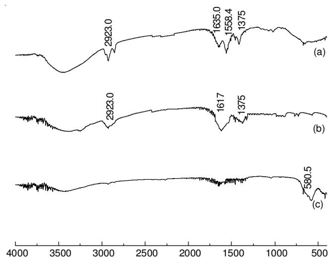
Fig. 1. FTIR spectra of samples: (a)  $\text{Co}_{0.5}\text{Mn}_{0.5}\text{Fe}_2\text{O}_4$ -chitosan nanoparticles, (b) chitosan nanoparticles, (c)  $\text{Co}_{0.5}\text{Mn}_{0.5}\text{Fe}_2\text{O}_4$  particles
