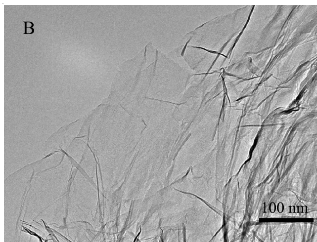
Fig. 1. (A) Cyclic voltammograms (CVs) of a graphene oxide-modified GCE in 0.1 mol/L KCl solution at a scan rate of 50 mV/s. (B) Typical TEM image of electrochemical reduction of graphene nanosheet electrochemical reduction of graphene oxide (EG)
