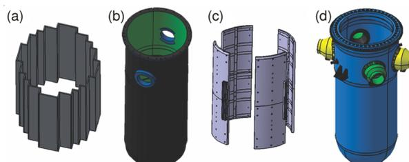
Fig. 1. Main components in reactor pressure vessel ((a) Baffle, (b) Barrel, (c) thermal shield, (d) vessel)
