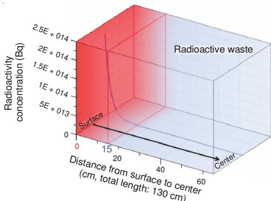
Fig. 3. Radioactivity concentration of radioactive waste by the distance
