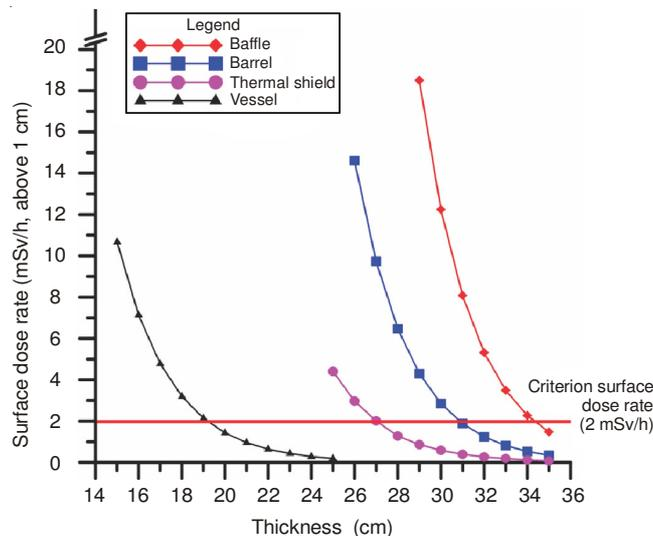
Fig. 2. Surface dose rate according to the thickness of main components
