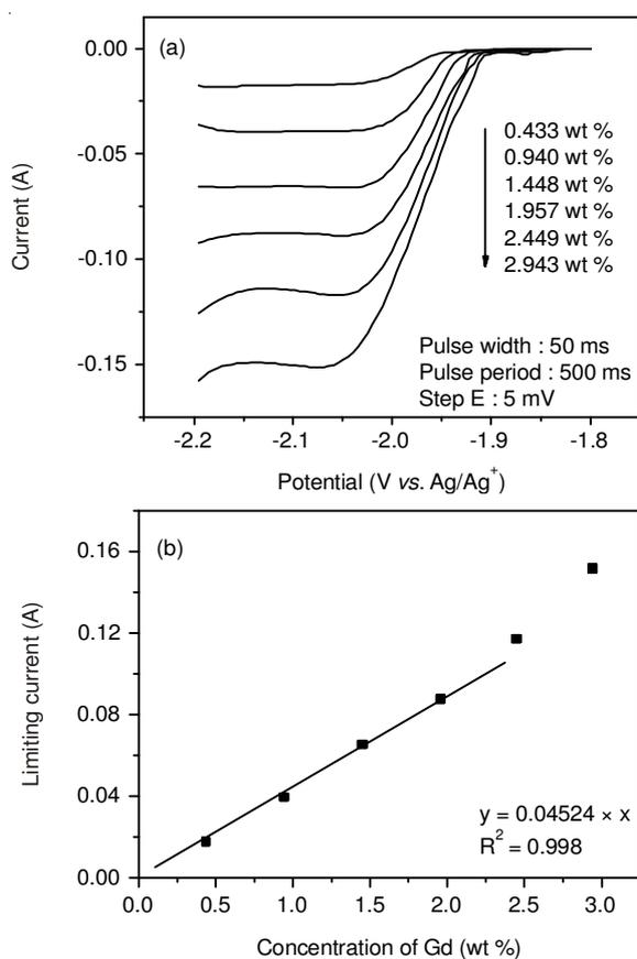
Fig. 3. (a) NPV curves obtained in various Gd(III) concentrations and (b) the plot of limiting current *versus* Gd(III) concentration and the calibration curve in the linear region
