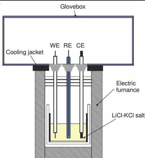
Fig. 1. A schematic of a high-temperature electrochemical cell in LiCl-KCl molten salts
