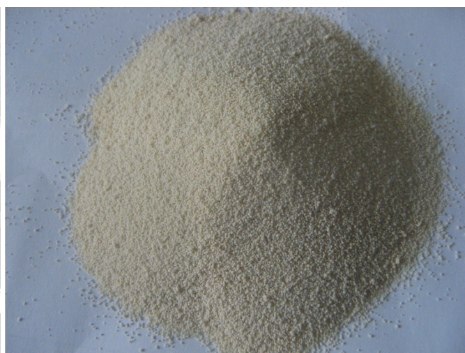
(b) Picture of spherical ammonium dinitramide (ADN)
