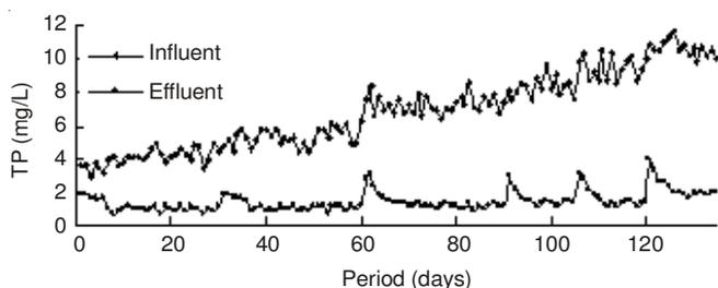
Fig. 4. Influent and effluent TP in different mixing ratios and organic load
