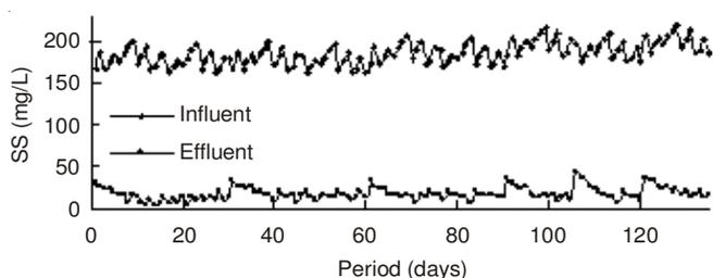
Fig. 5. Influent and effluent SS in different mixing ratios and organic loads
