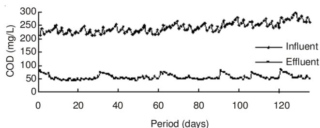
Fig. 2. Influent and effluent COD in different mixing ratios and organic load
