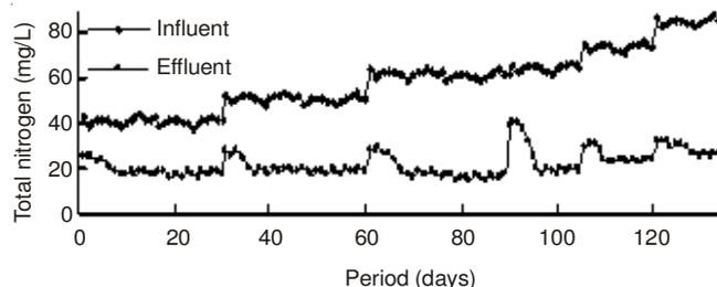
Fig. 3. Influent and effluent total nitrogen in different mixing ratios and organic load
