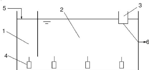
Fig. 1. Structure of CASS pool. 1-Pre-reaction zone 2-main reaction zone 3-decanter 4-aerator 5-influent 6-effluent
