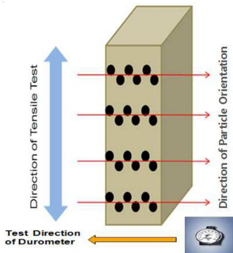
Scheme-II: Schematic diagram for the direction of particle orientation and test
