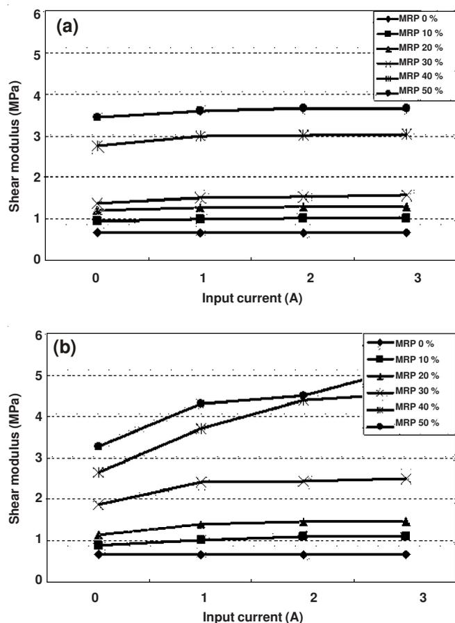
Fig. 5. Change of shear moduli of MREs according to input current : (a) i-MRE, (b) a-MRE
