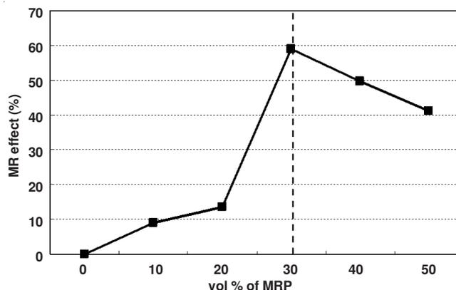
Fig. 6. Modified magneto-rheological effect of a-MRE compared with i-MRE
