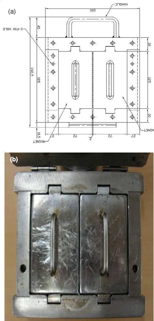
Fig. 1. Neodymium magnet inserted mold : (a) design drawing, (b) inside of real mold
