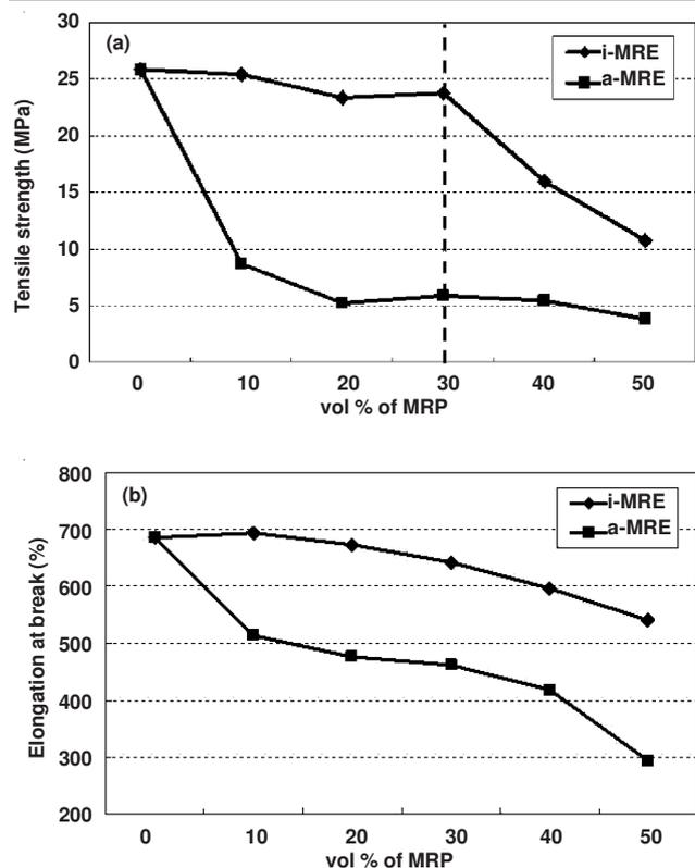
Fig. 3. Tensile properties of MRE with the amounts of magneto-responsive particles : (a) Tensile strength, (b) Elongation at break
