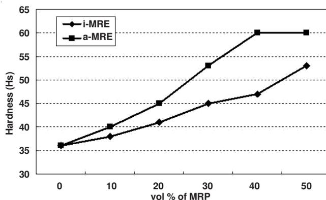
Fig. 4. Hardness of magneto-rheological elastomer with the amounts of magneto-responsive particles
