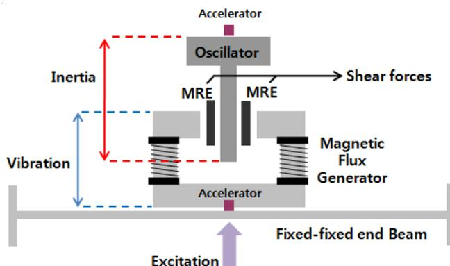
**Scheme-I:** Self-modified fast Fourier transform analyzer for measurement of shear modulus of magneto-rheological elastomer specimen
