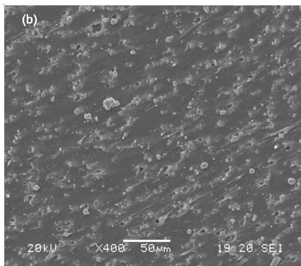
**Fig. 2.** Morphology of magneto-rheological elastomers with the type of manufacturing process: (a) i-MRE, (b) a-MRE
