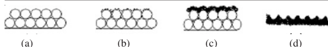
Fig. 1. (a) Ordered assembly of polystyrene nanoparticles as the template (b) Chemical assembly of Ag metal for few minutes (c) Chemical deposition of Ag metal for half hour (d) Removal of polystyrene particles
