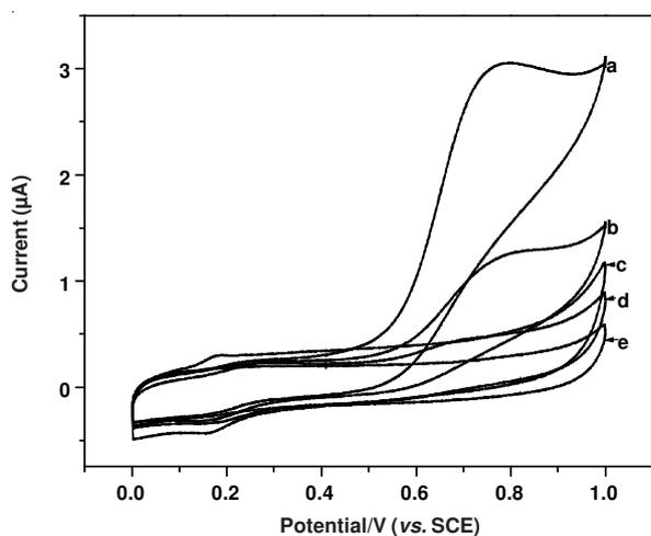
Fig. 2. Cyclic voltammograms of the AChE/CHIT-GO/GCE (a, e), AChE/GCE (b), GCE (c) and CHIT-GO/GCE (d) in 0.2 M PBS solution (pH 7.0) in the presence (a, b, c, d) and absence (e) of 0.4 mM ATCl. Scan rates:  $40 \text{ mV s}^{-1}$
