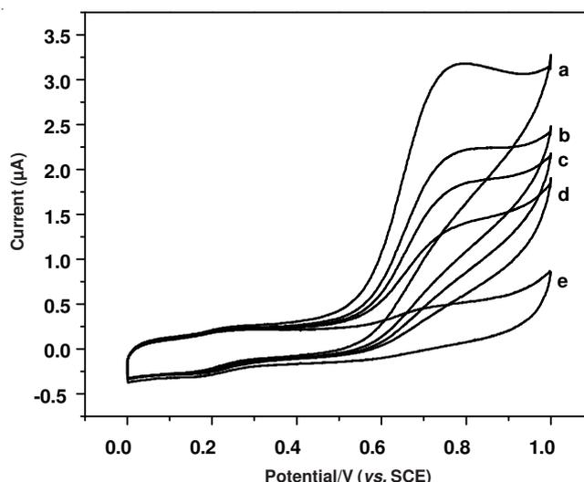
Fig. 4. Cyclic voltammograms of AChE/CHIT-GO/GCE in 0.2 M PBS solution (pH 7.0) containing 0.4 mM ATCl after adding different concentration of carbaryl: 0 (a), 0.2 (b), 0.3 (c), 1.0 (d) and 4.0 (e)  $\mu\text{M}$ . Scan rate:  $40 \text{ mV s}^{-1}$
