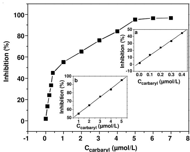
Fig. 5. Inhibition of AChE/CHIT-GO/GCE in 0.2 M PBS (pH 7.0) containing 0.4 mM ATCl after adding different concentration of carbaryl. Inset: calibration curves in the range of 0.005-0.4  $\mu\text{M}$  (A) and 1.0-5.0  $\mu\text{M}$  (B), respectively
