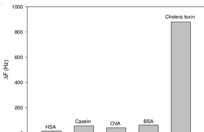
Fig. 8. Frequency of the developed biosensor to different proteins: HSA (10 mg/mL), casein (saturated solution in PBS), ovalbumin (saturated solution in PBS), BSA (10 mg/mL) and CT (100 ng/mL)
