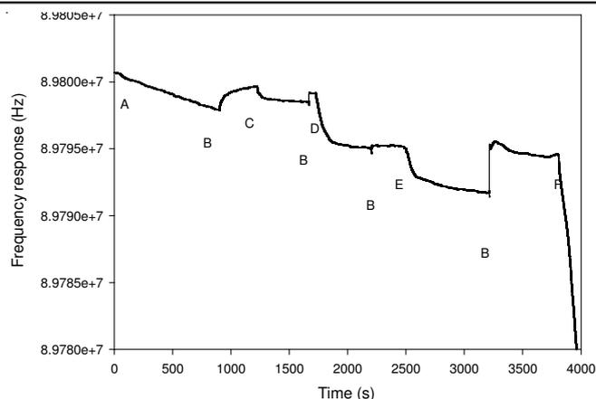
Fig. 2. Real-time interaction processes of the sensing surface in the determination of CT as monitored using microgravimetric QCM analysis
