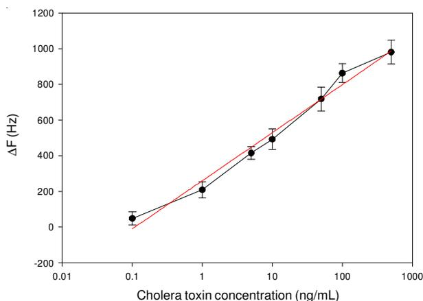
Fig. 7. Calibration curves of the relationship between the frequencies response and the concentration of cholera toxin. The red line describes the linear relationship between frequency responses (ΔF) vs. the logarithm of CT concentration
