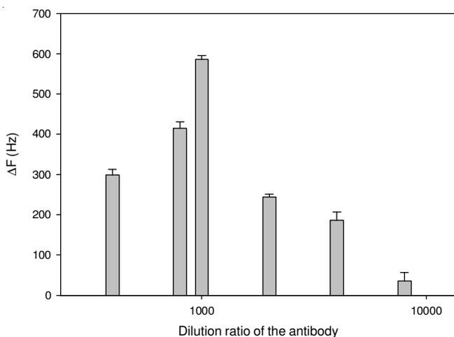
Fig. 4. Frequency responses of vary anti CT antibody dilution ratios in the assay medium (the sensor surfaces were incubated with GM1 tethered lipid membrane and had reacted with 2.5 μg/mL CT)
