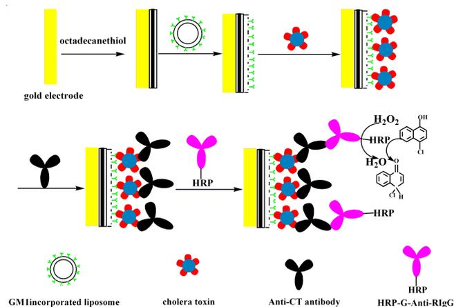
Fig. 1. Schematic diagram of the developed biocatalyzed deposition biosensor for cholera toxin
