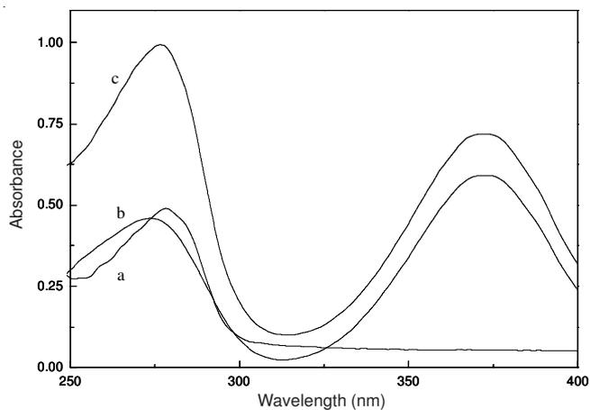
Fig. 5. UV-visible spectra of BSA (a), Cr(VI) (b) and BSA-Cr(VI) (c),  $c_{(\text{BSA})} = 1.0 \times 10^{-5} \text{ mol L}^{-1}$ ,  $c_{(\text{Cr(VI)})} = 1.0 \times 10^{-4} \text{ mol L}^{-1}$
