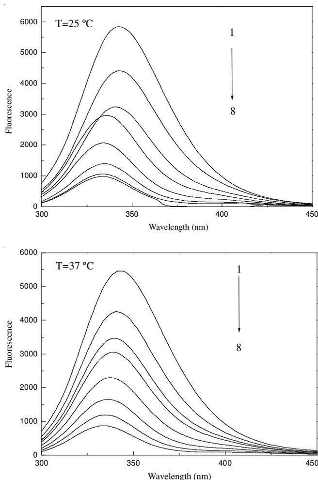
Fig. 1. Effect of Cr(VI) on quenching of BSA fluorescence (25 °C and 37 °C),  $c_{(BSA)} = 1.0 \times 10^{-5} \text{ mol L}^{-1}$ ,  $c_{(Cr(VI))}/10^{-4} \text{ mol L}^{-1}$ , 1 to 8: 0, 0.4, 0.8, 1.0, 1.6, 2.4, 3.2, 4.0
