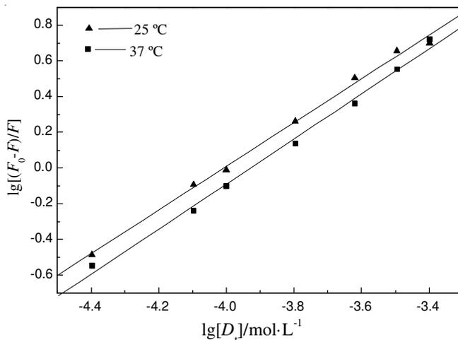
Fig. 3. Double-logarithm curves of BSA quenched by Cr(VI)
