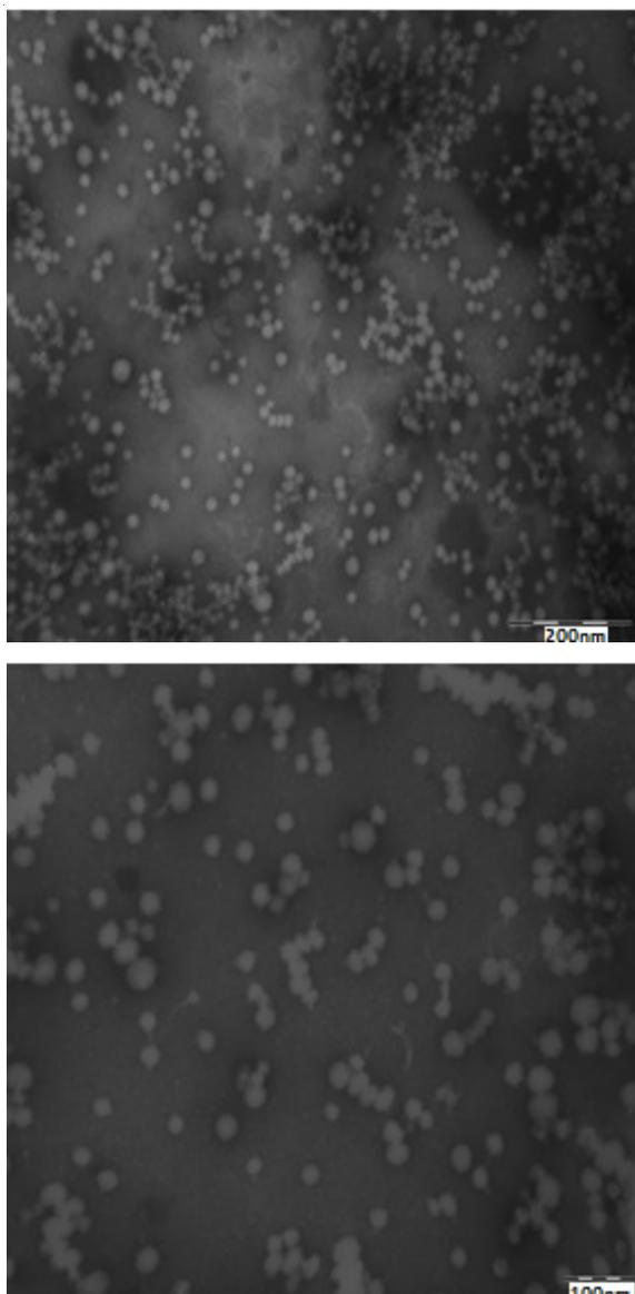
Fig. 2. Morphology of GB-PBCA nanoparticles observed by TEM [Top: nanoparticles solution ( $\times 70000$ ), bottom: redissolving solution of nanoparticles after lyophilization ( $\times 100000$ )]
