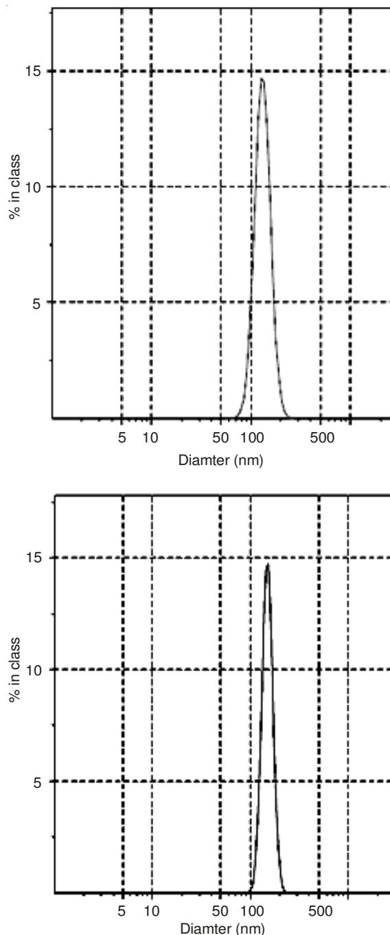
Fig. 3. Size distribution of the particles diameter of PBCA-GB (left: solution state; right: redispersion state)
