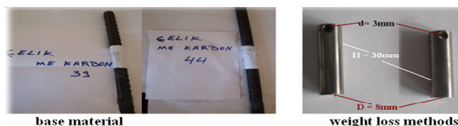
Fig. 2. Preparation of the samples for weight loss measurements
