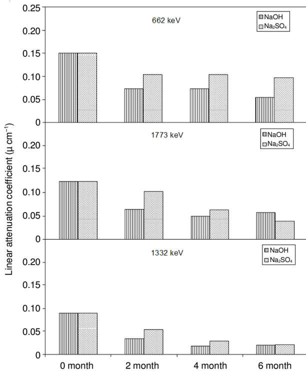
Fig. 4. Variation of the linear attenuation coefficients with the different chemical media obtained at 662, 1773 and 1332 keV energy
