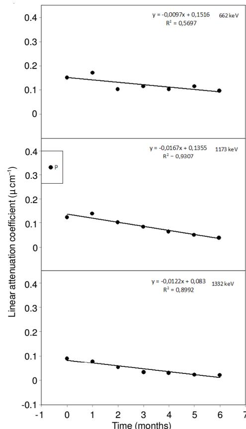
Fig. 3. Variation of the linear attenuation coefficients with the time for 662, 1773 and 1332 keV energy photons in Na<sub>2</sub>SO<sub>4</sub> medium
