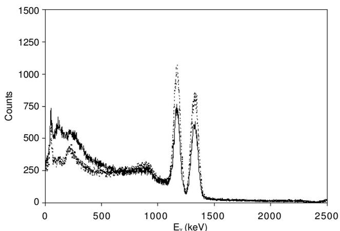
Fig. 1. Photon energy spectrum with and without concrete between detector and <sup>60</sup>Co radioactive source
