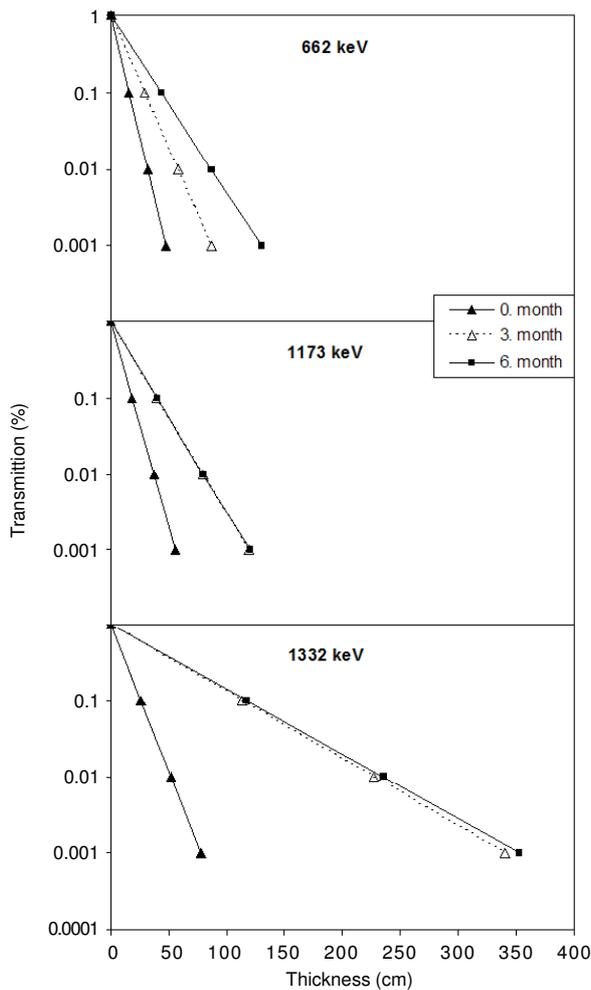
Fig. 5. Transmission rate of  $\gamma$ -rays at different energies for various month chemical effect in NaOH medium
