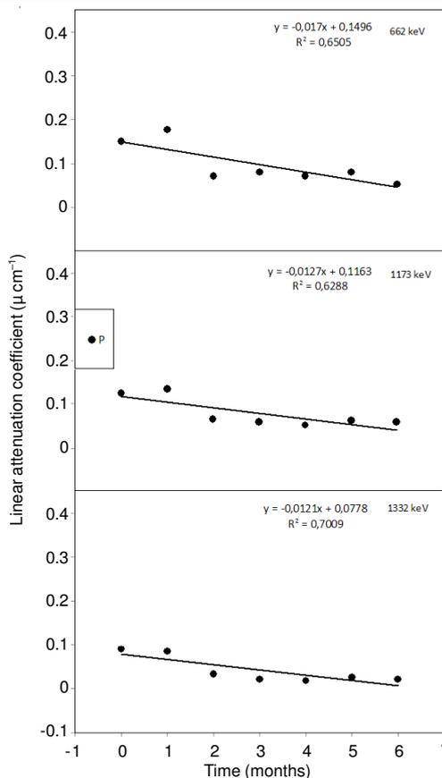
Fig. 2. Variation of the linear attenuation coefficients with the time for 662, 1773 and 1332 keV energy photons in NaOH medium
