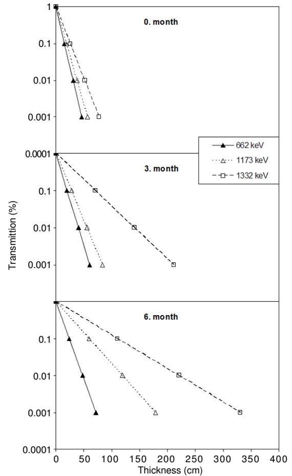
Fig. 6. Transmission rate of  $\gamma$ -rays at different energies for 662, 1173 and 1332 keV photon energies in Na<sub>2</sub>SO<sub>4</sub> medium
