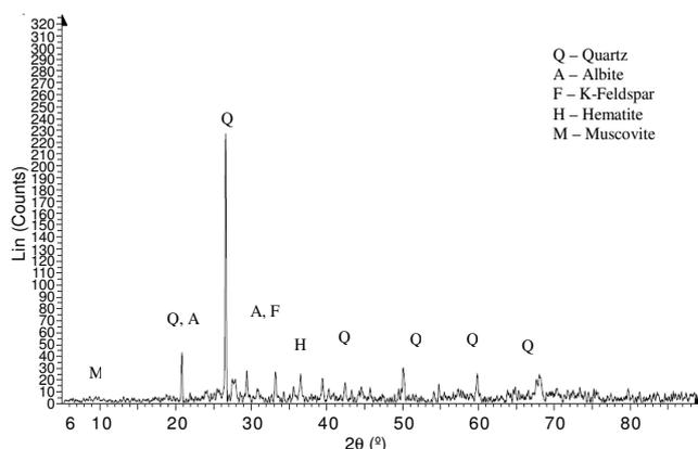
Fig. 3. XRD pattern of the Mughal brick sample (BSJT-1) with peaks of quartz, albite, feldspar, hematite and muscovite minerals
