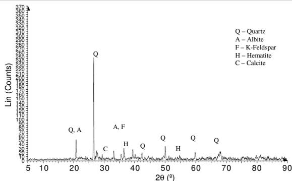
Fig. 4. XRD pattern of the Mughal brick sample (BSJT-4) with peaks of quartz, albite, feldspar, hematite and muscovite minerals with a very low peak for calcite
