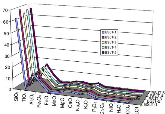
Fig. 5. The chemical composition (major elements) of Mughal bricks showing high amounts of SiO<sub>2</sub>, Al<sub>2</sub>O<sub>3</sub>, and Fe<sub>2</sub>O<sub>3</sub> with low amounts of Na<sub>2</sub>O, MgO and CaO from Jahangir Tomb
