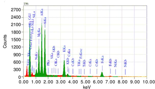
Fig. 7. Mughal Brick sample (a) BSE-SEM micrograph (b) EDS spectrum of brick sample showing high amounts of silica, alumina and iron oxide with low amounts of soda, potash, magnesia and negligible calcium oxide from Jahangir Tomb
