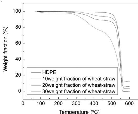
Fig. 3. TGA curves of different wheat straw contents
