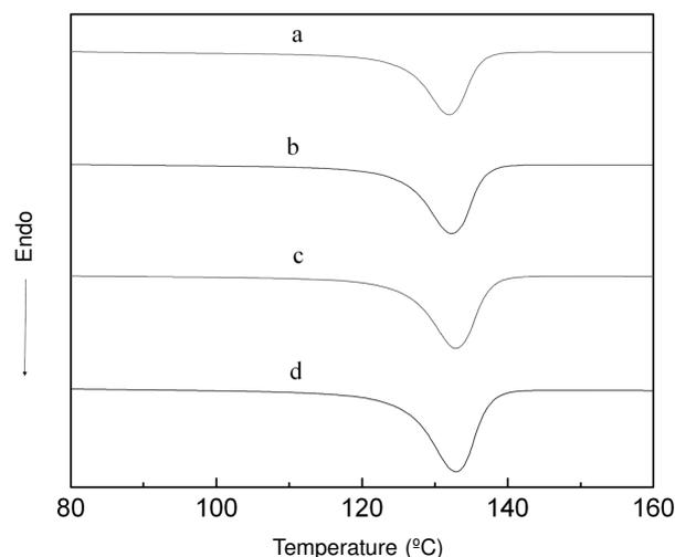
Fig. 2. DSC curves of different wheat straw contents, and the wheat-straw weight fraction a (30 %), b (20 %), c (10 %), d (0)
