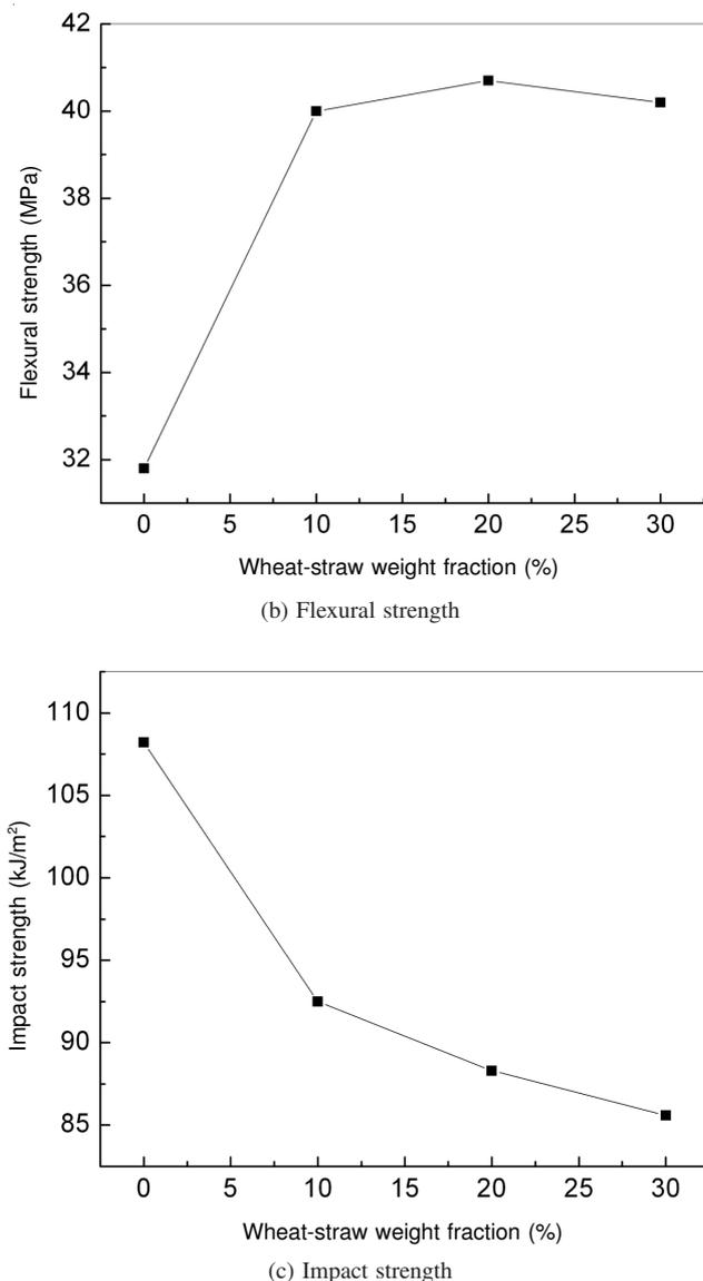
Fig. 4. Mechanical properties of different wheat straw flour percents
