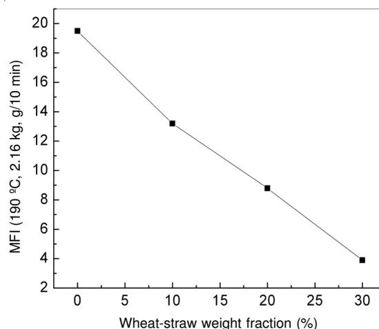
Fig. 1. Fluidity of the composites with the content of wheat-straw
