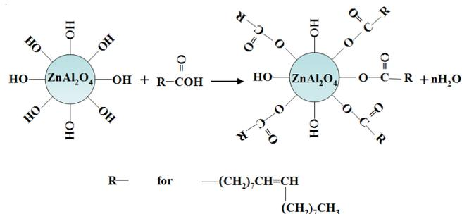
Fig. 3. Scheme of the oleic acid grafting on the solid surface of ZnAl<sub>2</sub>O<sub>4</sub>
