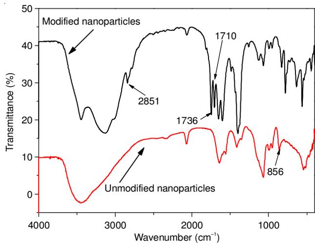
Fig. 4. FTIR spectra of unmodified and modified ZnAl<sub>2</sub>O<sub>4</sub> nanoparticles
