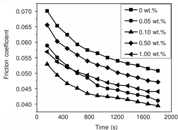
Fig. 6. Friction coefficient curve with time tested with different concentration of ZnAl<sub>2</sub>O<sub>4</sub>
