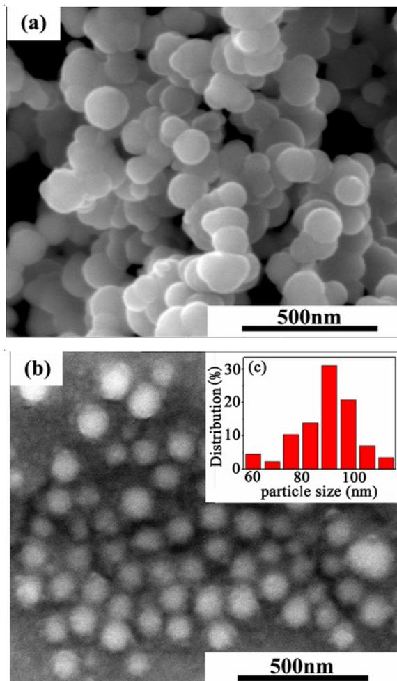
Fig. 2. TEM photographs of  $\text{ZnAl}_2\text{O}_4$  particles (a) unmodified, (b) modified, (c) Size histograms of  $\text{ZnAl}_2\text{O}_4$  nanoparticles
