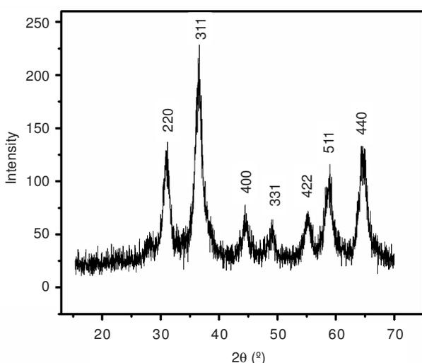
Fig. 1. XRD pattern of  $\text{ZnAl}_2\text{O}_4$  nanoparticles
