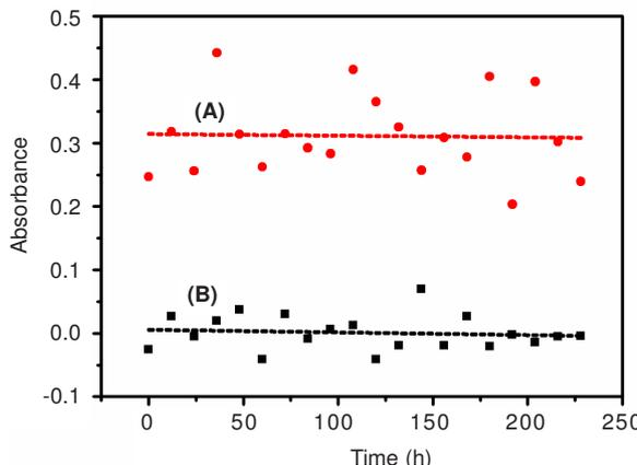
Fig. 5. Absorbance-time scatter of (a) oil (b) oil . with 1 wt % ZnAl<sub>2</sub>O<sub>4</sub> nanoparticles
