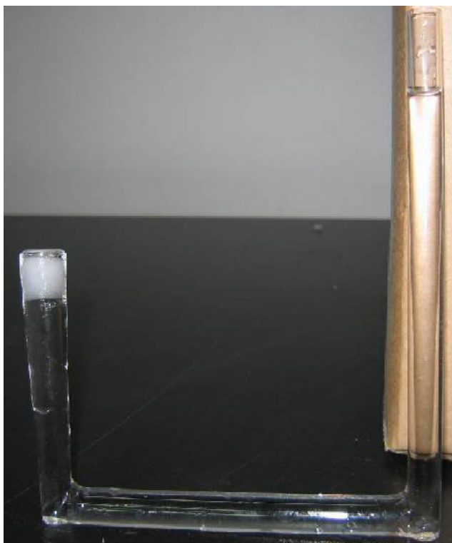
Fig. 3. 16 mm long ice achieved in the left side of the crucible
