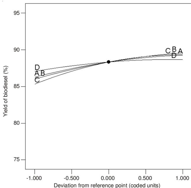
Fig. 2. Perturbation plot of the reaction parameters. (A) Catalyst loading, (B) Methanol/oil molar ratio, (C) Reaction temperature and (D) reaction time
