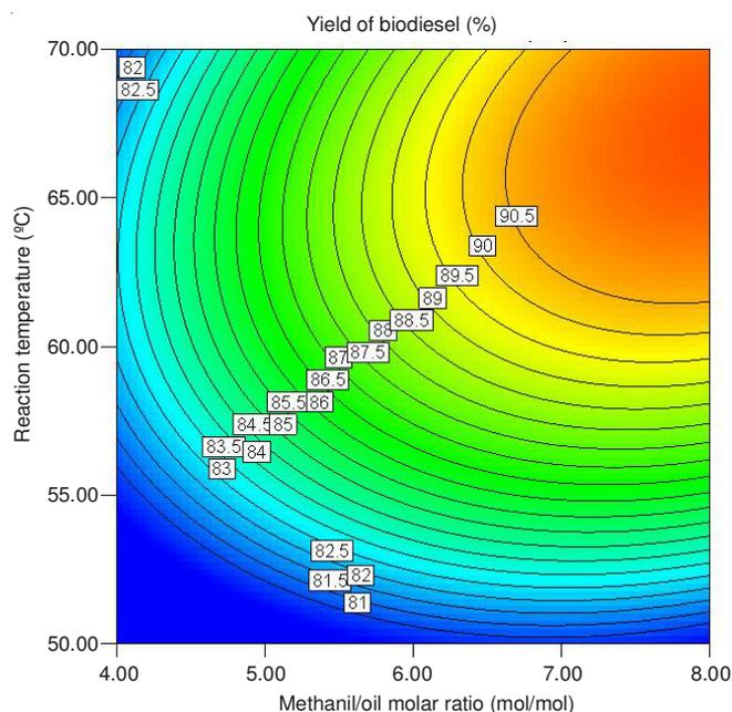
Fig. 4. Contour plot of the effect of methanol/oil molar ratio and reaction temperature on methyl esters yield
