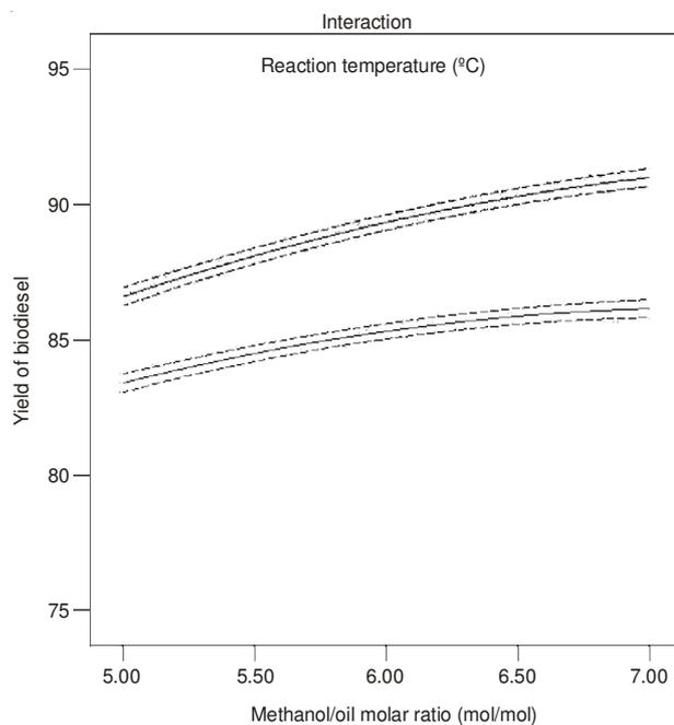
Fig. 3. Two-dimensional plot of the effect of methanol/oil molar ratio and reaction temperature on methyl esters yield
