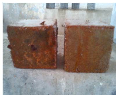
Specimens after immersing in \text{HNO}_3
