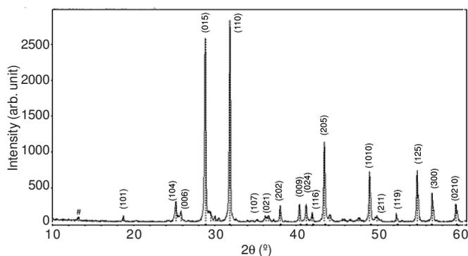
Fig. 2. XRD patterns of the  $\text{Sr}_3\text{V}_2\text{O}_8$  nanoparticles synthesized
