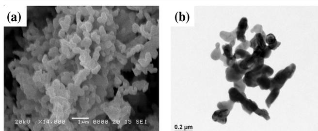
Fig. 3. SEM image (a) and TEM image (b) of the  $\text{Sr}_3\text{V}_2\text{O}_8$  nanoparticles
