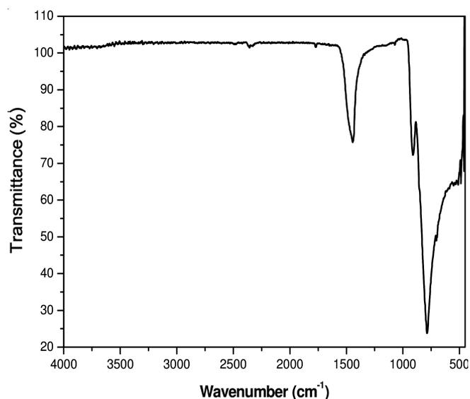
Fig. 4. FT-IR spectrum of the  $\text{Sr}_3\text{V}_2\text{O}_8$  nanoparticles synthesized
