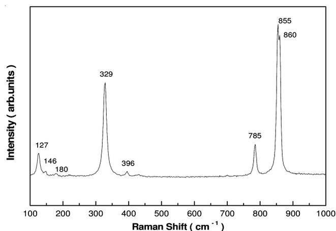
Fig. 6. Raman spectrum of the synthesized  $\text{Sr}_3\text{V}_2\text{O}_8$  nanoparticles excited by the 514.5 nm line of an Ar-ion laser at 0.5 mW on the samples
