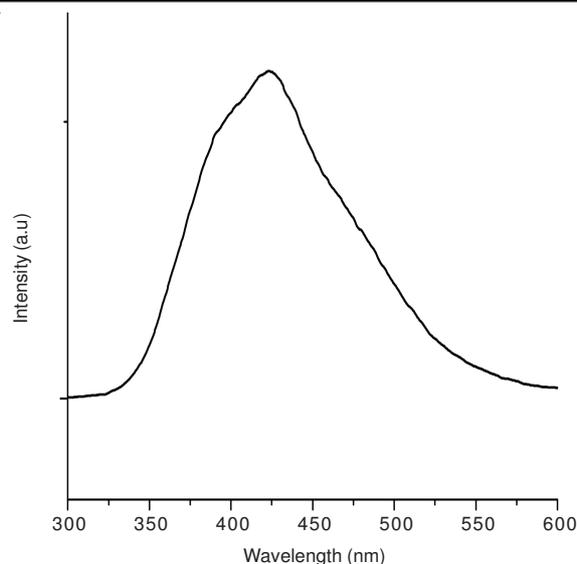
Fig. 5. Photoluminescence emission spectrum of the synthesized  $\text{Sr}_3\text{V}_2\text{O}_8$  nanoparticles excited at 250 nm at room temperature
