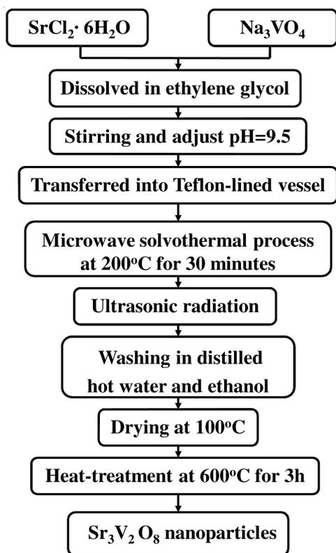
Fig. 1. Flow chart for the synthesis of  $\text{Sr}_3\text{V}_2\text{O}_8$  nanoparticles by the microwave solvothermal process
