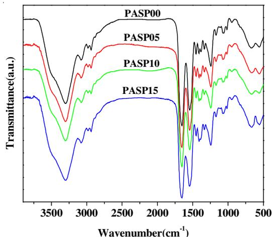
Fig. 1. FT-IR spectra of SF/PASP in different proportions before electro-spinning
