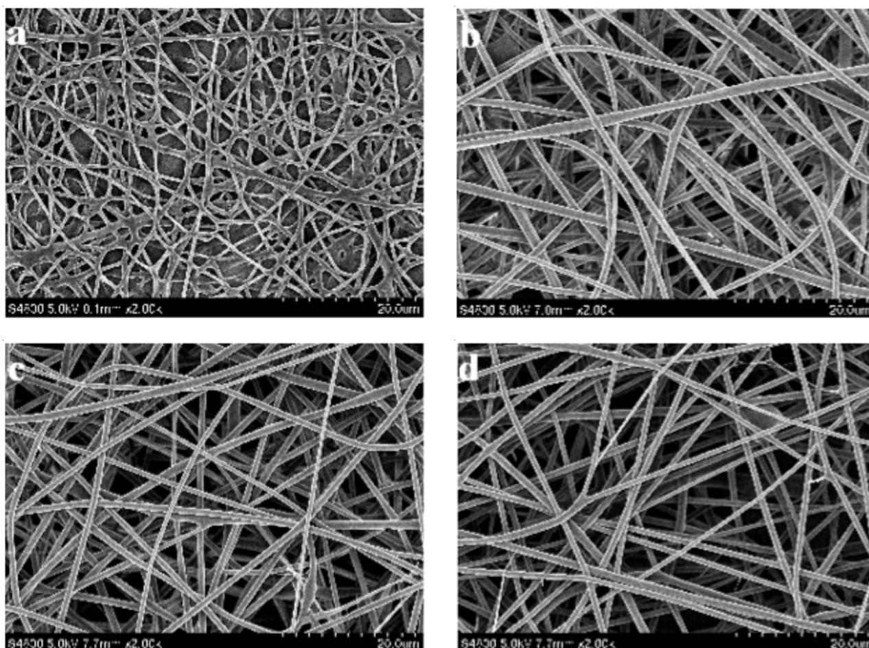
Fig. 5. Scanning electron microscopy of PASP/SF scaffolds (a) PASP00, (b) PASP05, (c) PASP10, (d) PASP15
