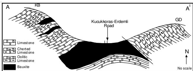
Fig. 10. Horizontal geological sections of Uctepeler formation around the village Kucukkoras and bauxite reserves
