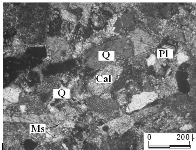
Fig. 5. A general view of meta-sandstones. Q: quartz, Pl: plagioclase, Ms: muscovite, Cal: calcite (double nicol)
