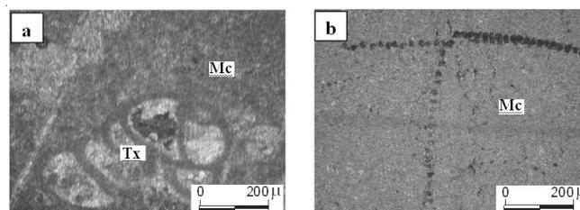
Fig. 8. Thin sections of Uctepeler limestone: (a) Micrite (Mc) and textularidae (Tx) in biomicrite (single nicol), (b) Micrite (Mc) and radiolaria va tintinitler in biomicrite (single nicol)
