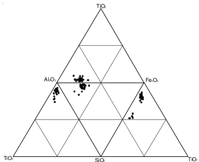
Fig. 15. Triangular diagrams of Kucukkoras bauxite specimens based on their major oxide compositions
