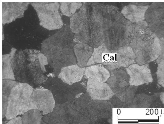
Fig. 7. View of crystallized limestone from uctepeler formation. Cal: calcite (double nicol)
