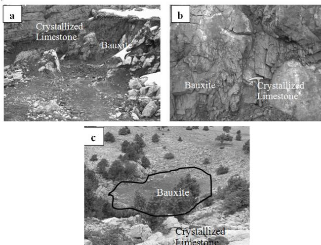
Fig. 9. Bauxite reserves in Uctepeler formation in the mines on Mihliardic Ridges (a) Bauxite in crystallized limestone, (b) Bauxite filling the spaces of crystallized limestones, (c) Bauxites in the Dolines in Korkuyu in the southeast of Mihliardic ridge
