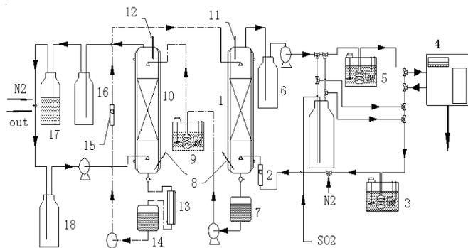
Fig. 1. Sketch of GLE experimental apparatus. 1 Absorption tower; 2, 15 Flowmeter; 3, 5, 9 Thermostatted bath; 4 GC; 6, 7, 14, 16, 17, 18 Buffer; 8, 11, 12 Thermometer; 10 Desorption tower; 13 Cooler
