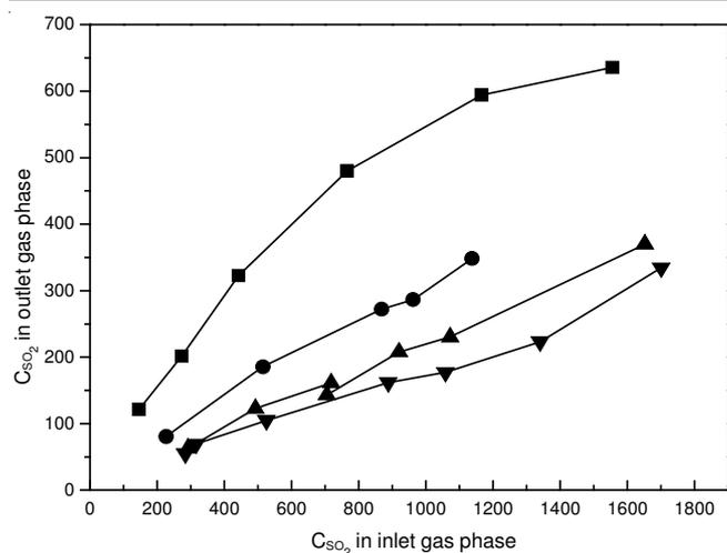
Fig. 2.  $\text{SO}_2$  concentrate relation between inlet gas and outlet gas at various gas-liquid ratio: ■  $G/L = 20$  ●  $G/L = 10$  ▲  $G/L = 7.5$  ▼  $G/L = 3$
