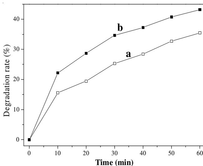
Fig. 6. Degradation of ciprofloxacin and gatifloxacin with ZnS under visible light irradiation
