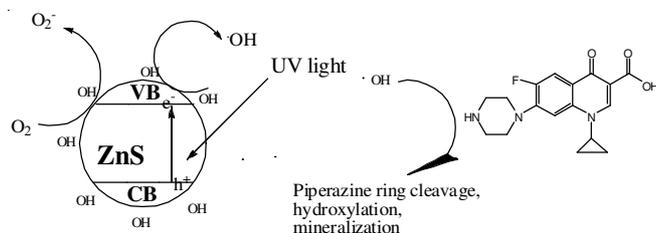
Fig. 7. Scheme of degradation ciprofloxacin with ZnS photocatalyst
