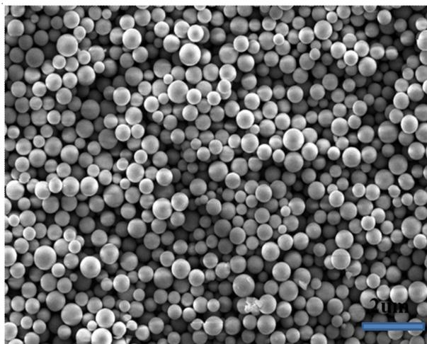
Fig. 4. SEM of prepared ZnS
