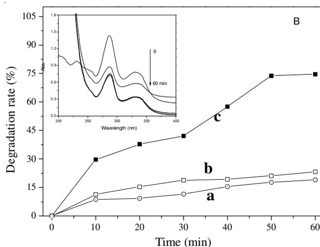
Fig. 5. Degradation of ciprofloxacin (A) and gatifloxacin (B) with ZnS under UV light irradiation
