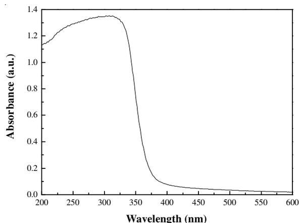
Fig. 1. UV-VIS of prepared ZnS
