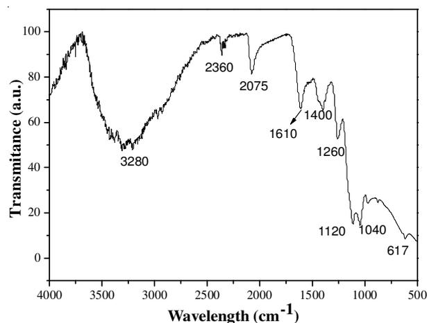
Fig. 3. FT-IR of prepared ZnS sample
