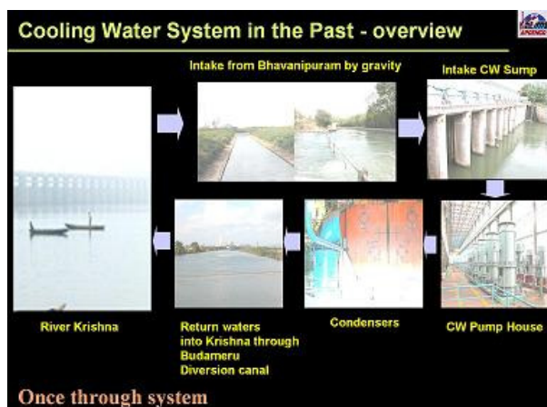
Fig. 4. Over view of the in-taking and out letting water of Vijayawada thermal power station
