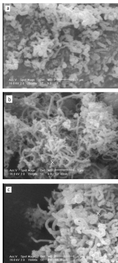
Fig. 4. SEM images of synthesized carbon nanotubes on Fe\* (nm)/Al<sub>2</sub>O<sub>3</sub> under different growth temperatures; (a) 865 °C, (b) 925 °C and (c) 975 °C
