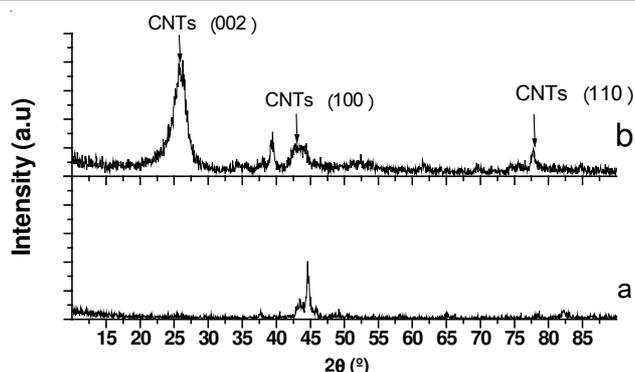
Fig. 2. XRD Patterns of Fe nanoparticles powder without any support (a) and CNTs synthesized on Fe catalyst in 925 °C (b)
