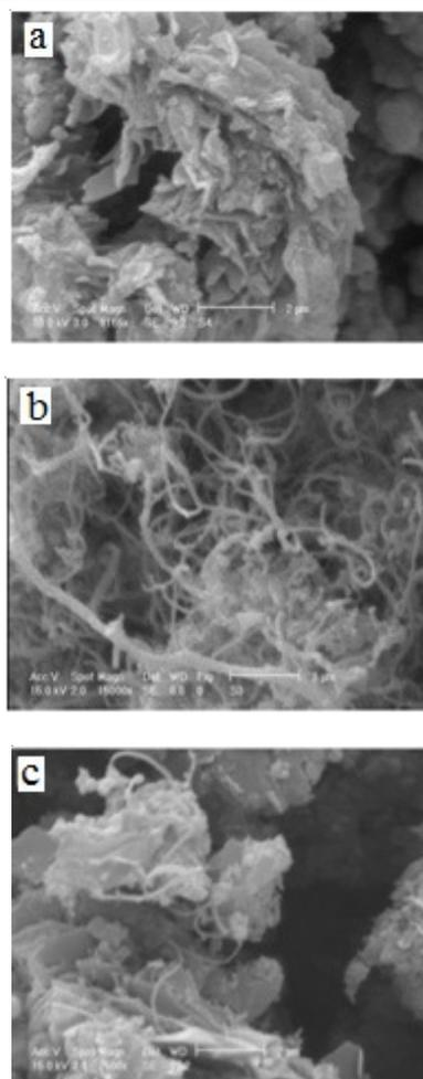
Fig. 1. SEM images of catalytic decomposition of ethylene on Fe nanoparticles without used supports at; (a) 865 °C, (b) 925 °C and (c) 975 °C
