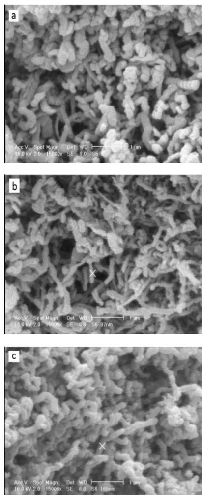
Fig. 5. SEM images of synthesized CNTs on Fe\* (nm)/MgO under different growth temperatures; (a) 865 °C, (b) 925 °C, and (c) 975 °C
