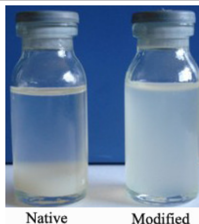
Fig. 5. Image of oil-soluble about nano-oil with nanoparticles
