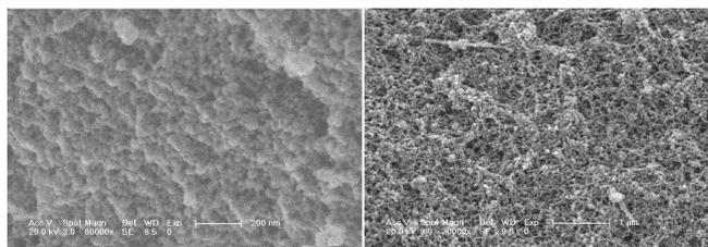
Fig. 4. SEM photographs of pure silica aerogel (left) and reinforced silica aerogel doped with fibrous brucite (right)
