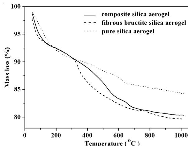
Fig. 2. TGA curves of silica aerogels samples
