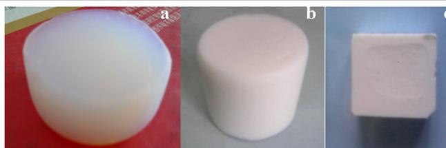
Fig. 1. Photographs of silica aerogels samples
