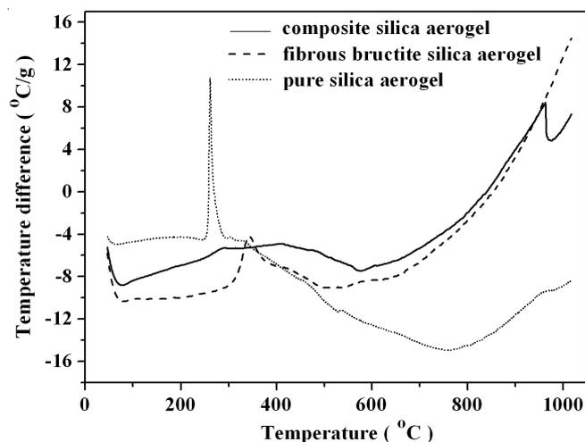
Fig. 3. DTA curves of silica aerogels samples
