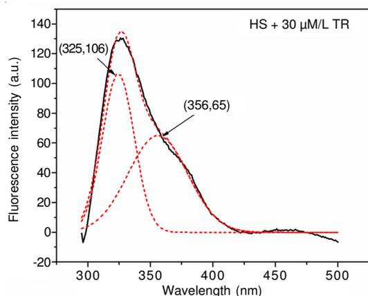
Fig. 6. Guassion fitting of fluorescence spectra excited at 290 nm
