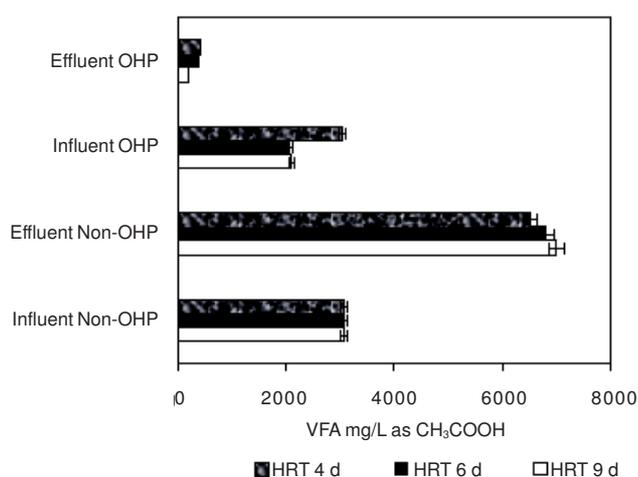
Fig. 3. Volatile fatty acid of effluent when operating continuous stirred tank reactor with oxidation by hydrogen peroxide and non-OHP petrochemical waste water at cycle time 12 h and hydraulic retention time 9, 6 and 4 days
