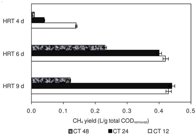
Fig. 5. Effects of co-digestion on oxidation by hydrogen peroxide pretreated petrochemical waste water in terms of CH<sub>4</sub> yield
