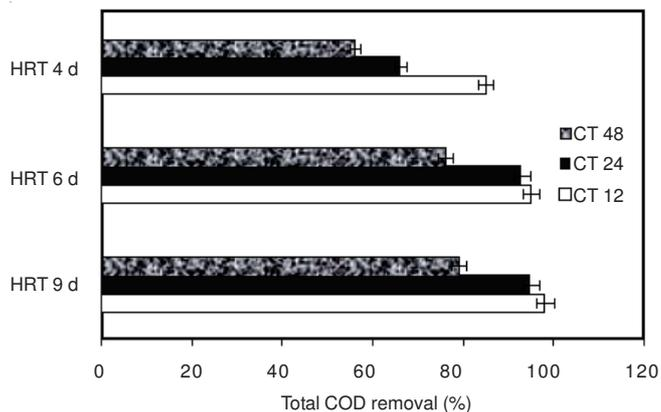
Fig. 4. Effects of co-digestion on oxidation by hydrogen peroxide pretreated petrochemical waste water in terms of total COD removal
