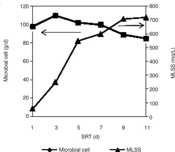
Fig. 7. Effluent microbial cell concentration vs. solid retention time for co-digestion process.
