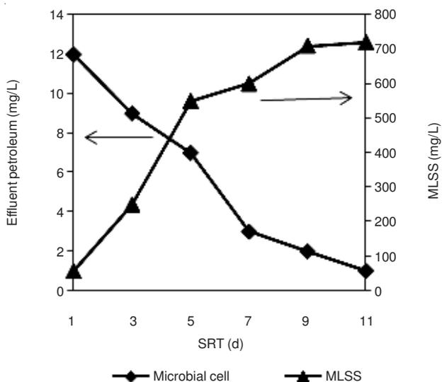
Fig. 6. Effluent petroleum concentration vs. solid retention time for co-digestion process
