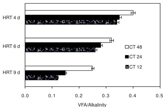
Fig. 1. Effects of co-digestion on oxidation by hydrogen peroxide pretreated petrochemical waste water in terms of volatile fatty acid/alkalinity ratio
