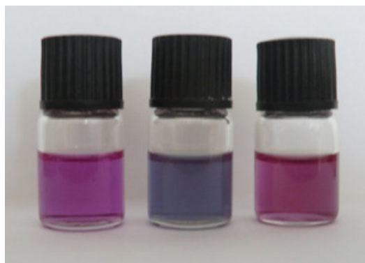
Fig. 2. Photograph of MgTPP (left), MgTPP + ethylenediamine (middle) and MgTPP + ethylenediamine + CO 2 (right)
