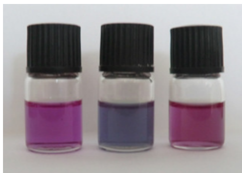
Fig. 2. Photograph of MgTPP (left), MgTPP + ethanolamine (middle) and MgTPP + ethanolamine + SO 2 (right)
