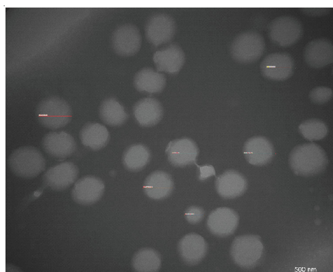
tungstic acid dyeing. After the emulsion adhesive is dyed by phosphotungstic acid, latex particle morphology is observed by transmission electron microscope. As is shown in Fig. 4, the emulsion particles has a dyed crust, center area is brighter than the edge and the obvious core-shell structure of emulsion particles is clearly shown by photographs. This is the same as the aforementioned DSC analysis results.
