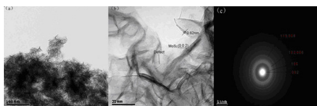
Fig. 2. (a) TEM image of MoS 2 -A3; (b) TEM image of MoS 2 -A3; (c) Electron diffraction pattern of MoS 2 -A3
