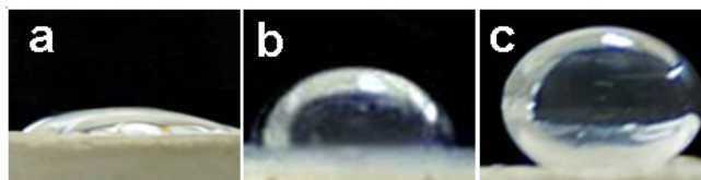
Fig. 6. Three-phase contact angle determination photograph of (a) SiO 2 , (b) SM2, (c) SM5
