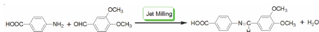
Scheme-I: Synthesis of Schiff base derived from 3,4-dimethoxybenzaldehyde and p -aminobenzoic acid
