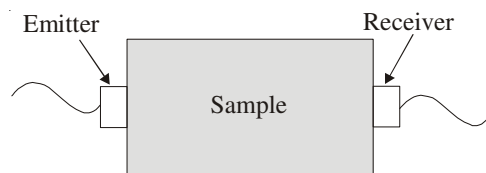
Fig. 2. Method of measuring P-wave velocity
