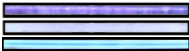
Fig. 3. Photograph of dielectric barrier discharge at atmospheric pressure in quartz tube. (a) Air; (b) argon; (c) argon/acetone
