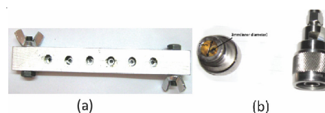
Fig. 1. (a) Device for the preparation of toroidal shape. (b) Waveguide (inner diameter 3 mm and outer diameter 7mm)
