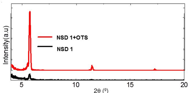
Fig. 4. Representative X-ray diffraction patterns of a 50 nm pentacene film deposited on : a) NSD 1 nanoscopic dielectric and b) NSD 1+OTS nanoscopic dielectric. The peak correspond to  $d = 15.5$  Å
