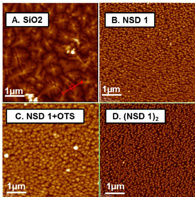
Fig. 3. Tapping mode AFM images ( $5 \times 5$  μm scan area) for morphology evaluation of 50 nm pentacene film grown at room temperature on the each nanoscale dielectric substrates. (A. 300 nm thick SiO<sub>2</sub>, B. NSD1, C. NSD 1 + OTS, D.  $[\text{NSD1}]_2$ )
