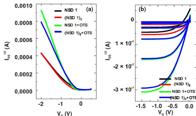
Fig. 5. Representative pentacene FET device performance at low bias with each nanoscale dielectric on n<sup>+</sup>-silicon gate (L/W = 100/1000 μm). (a) FET transfer plot of  $[I_{SD}]^{1/2}$  vs.  $V_G$  at  $V_{SD} = -2$  V. B. Current-voltage output plot as a function of  $V_G$  at  $V_{SD} = -1.5$  V
