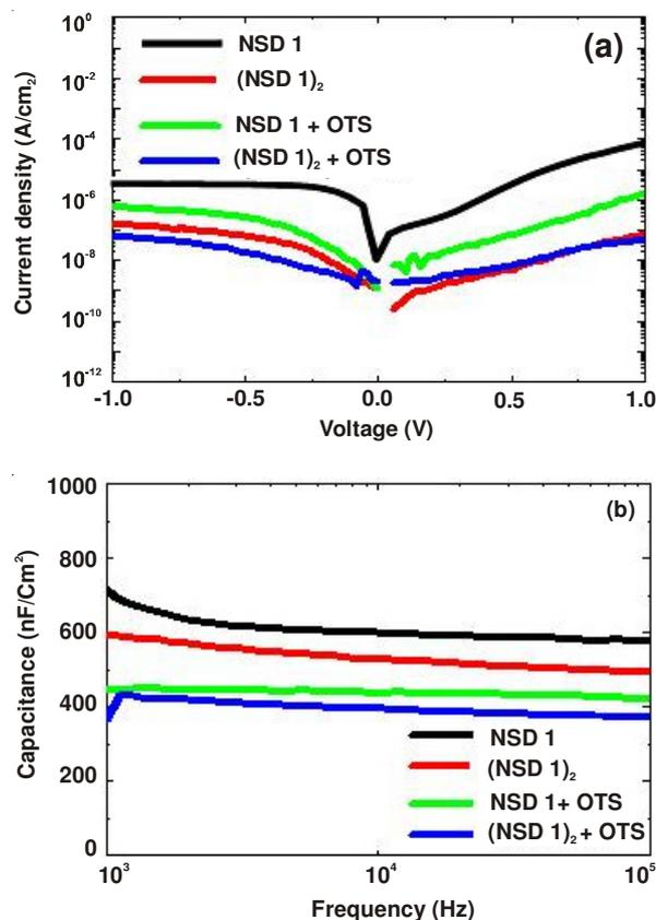
Fig. 2. (a) Measured leakage current density ( $J$ ) vs. voltage (V) plots with nanoscale dielectric (NSD1,  $[\text{NSD } 1]_2$ , NSD1 + OTS and  $[\text{NSD } 1]_2$  + OTS) in MIS sandwich structures on  $n^+$ -Si. (b) Capacitance vs. frequency (C-f) dependence of the capacitance in the accumulation regime (1 V) for each nanoscale dielectric in metal-insulator-semiconductor devices
