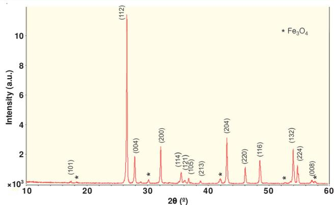
Fig. 1. XRD pattern of the synthesized  $\text{Fe}_3\text{O}_4$  incorporated  $\text{BaMoO}_4\cdot\text{Er}^{3+}/\text{Yb}^{3+}$  composites
