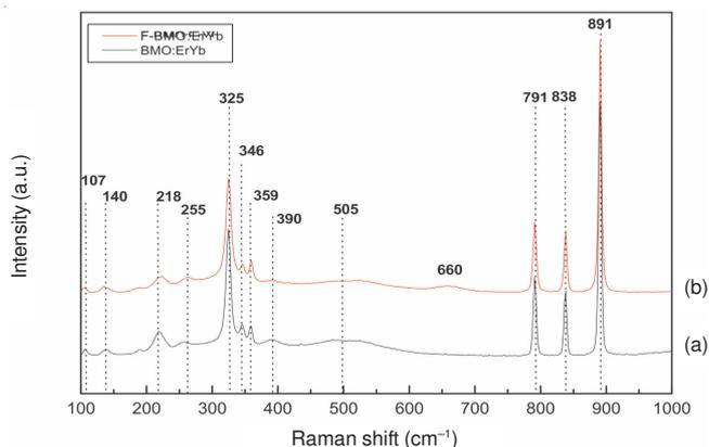
Fig. 5. Raman spectra of the synthesized (a)  $\text{BaMoO}_4:\text{Er}^{3+}$  (BMO:ErYb) particles and (b)  $\text{Fe}_3\text{O}_4$  incorporated  $\text{BaMoO}_4:\text{Er}^{3+}/\text{Yb}^{3+}$  (F-BMO:ErYb) composites excited by the 514.5 nm line of an Ar-ion laser at 0.5 mW on the samples
