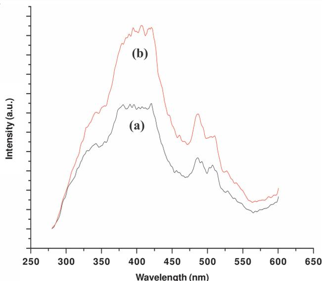
Fig. 4. Photoluminescence emission spectra of the synthesized (a) Fe<sub>3</sub>O<sub>4</sub> incorporated BaMoO<sub>4</sub>:Er<sup>3+</sup> and (b) Fe<sub>3</sub>O<sub>4</sub> incorporated BaMoO<sub>4</sub>:Er<sup>3+</sup>/Yb<sup>3+</sup> composites excited at 250 nm at room temperature
