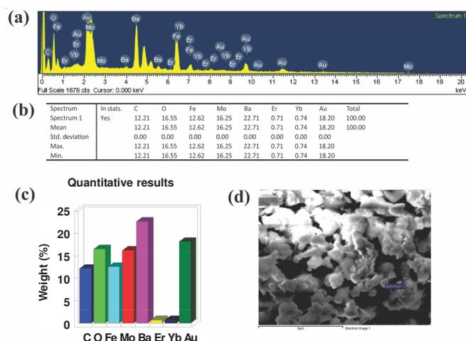
Fig. 3. (a) EDS pattern, (b) quantitative compositions, (c) quantitative results and (d) SEM image of the synthesized Fe<sub>3</sub>O<sub>4</sub> incorporated BaMoO<sub>4</sub>:Er<sup>3+</sup>/Yb<sup>3+</sup> composites
