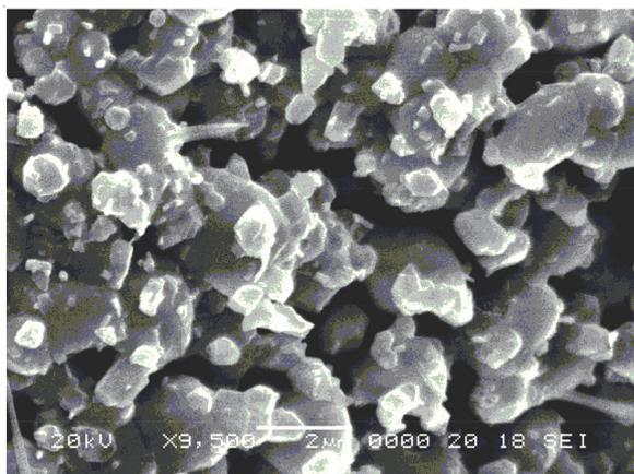
Fig. 2. SEM image of the synthesized Fe<sub>3</sub>O<sub>4</sub> incorporated BaMoO<sub>4</sub>:Er<sup>3+</sup>/Yb<sup>3+</sup> composites
