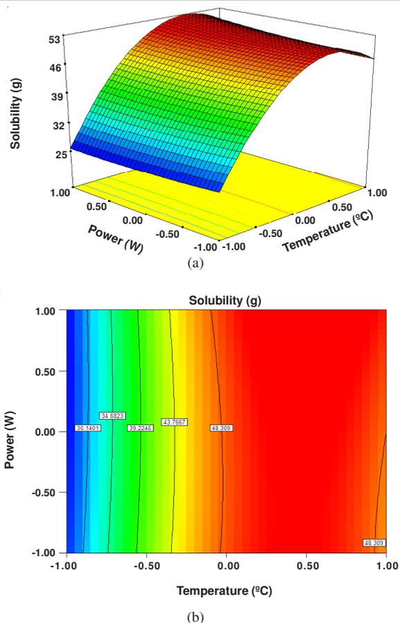
Fig. 6. 3D plot and contour plot of the effect of the independent variables temperature and power on solubility
