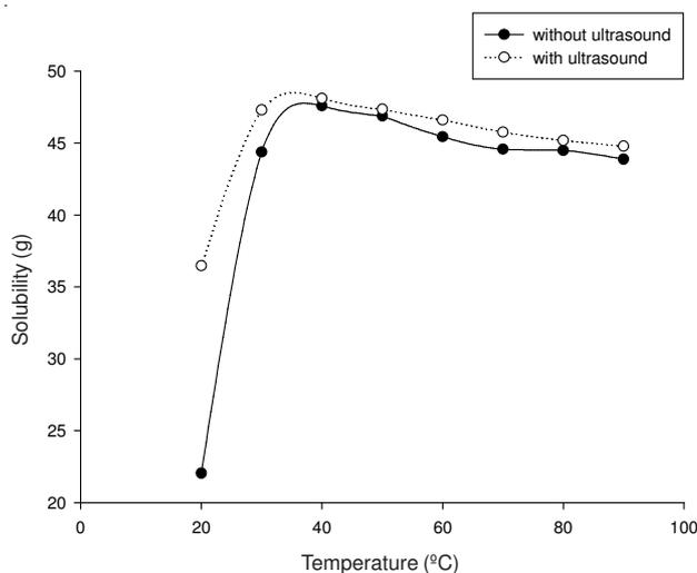
Fig. 1. Effect of temperature on the solubility with ultrasound and without ultrasound
