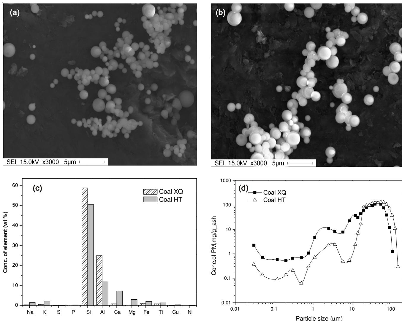
Fig. 3. Physical and chemical properties of PM<sub>2.5</sub> collected during single coal combustion. (a) SEM image of PM<sub>2.5</sub> formed from coal XQ; (b) SEM image of PM<sub>2.5</sub> formed from coal HT; (c) elemental composition of PM<sub>2.5</sub> produced from coals XQ and HT; (d) total size distribution of PM produced from coals XQ and HT
