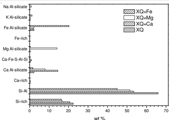
Fig. 6. A comparison of the mineral species in PM<sub>2.5+</sub> emitted from the combustion of coal XQ and HT
