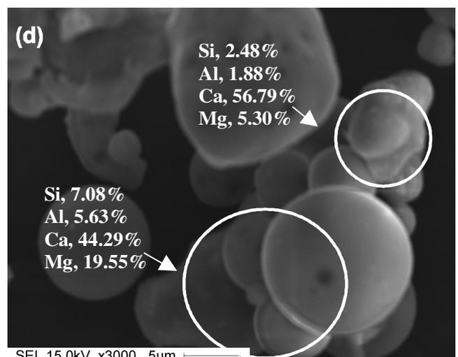
Fig. 5. SEM images of Al-Si and Ca-Mg-Al-Si in PM<sub>2.5+</sub>: (a and b) from XQ coal; (c and d) from HT coal
