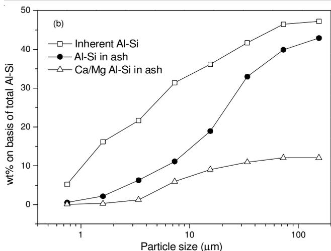
Fig. 4. Transformation of Al-silicate minerals ((a) for the inherent Al-Si in coal XQ and Al-Si in ash generating from coal XQ combustion and (b) for the inherent Al-Si in coal HT and Al-Si and Ca/Mg Al-Si in ash generating from coal combustion)
