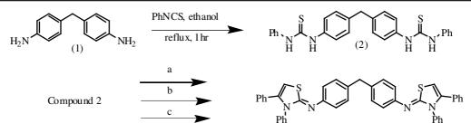
(a) Phenacylbromide (5mmol acetophenone, KBr & KBrO<sub>3</sub> (2:1, 1g, 5mmol available  $Br_2$ ), 1N HCl),  $I_2$ , DMF, reflux, overnight; (b) acetophenone,  $I_2$ , ethanol, reflux, 2hrs; (c) acetophenone,  $I_2$ , ethanol, ultrasonication, 30 mins
