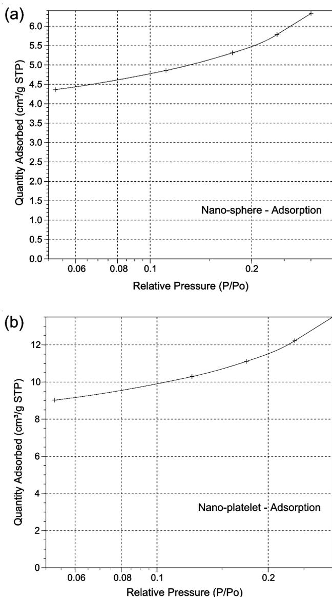
Fig. 5. Adsorption isotherm plot of MoS<sub>2</sub>: (a) nano-spheres and (b) nano-platelets
