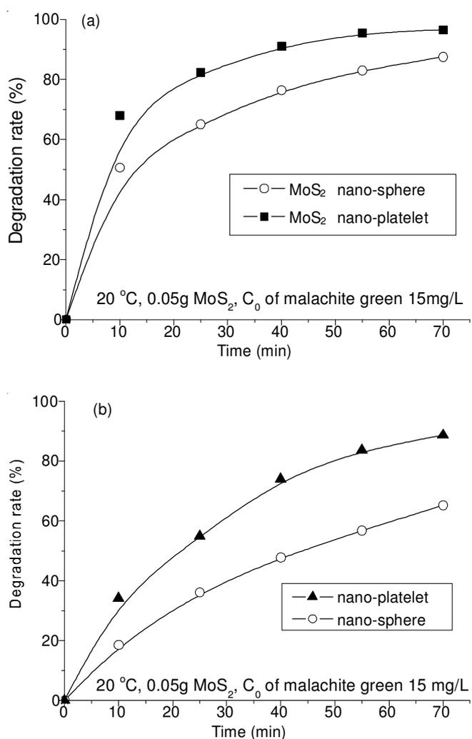
Fig. 4. Catalytic activity of 0.1 g MoS<sub>2</sub> used for (a) the 1<sup>st</sup> cycle and (b) the 4<sup>th</sup> cycle
