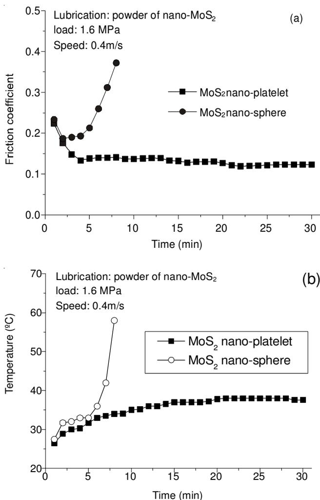
Fig. 3. Results of end-face tests: (a) friction coefficient and (b) friction temperature
