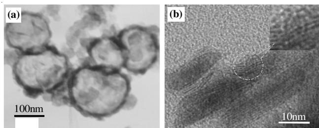
Fig. 2. Micrographs of (a) nano-spheres and (b) nano-platelets
