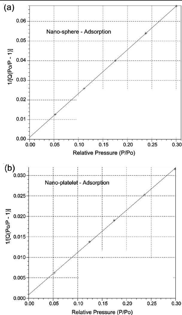
Fig. 6. BET surface area plot of MoS<sub>2</sub>: (a) nano-spheres and (b) nano-platelets
