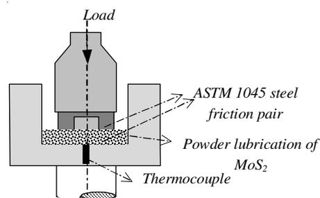
Fig. 1. Schematic diagram of the end-face tribological test
