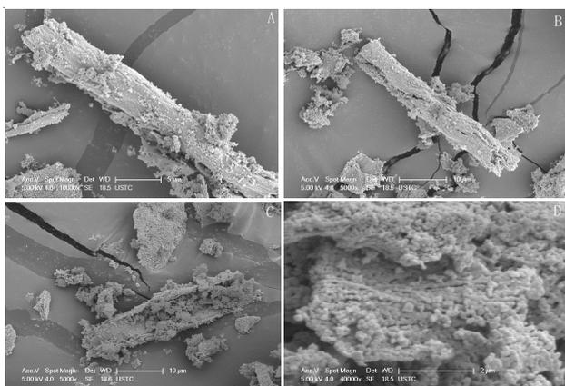
Fig. 2. SEM images of the  $\text{Zn}_{0.5}\text{Ni}_{0.5}\text{Fe}_2\text{O}_4$  microtubules
