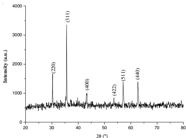
Fig. 1. XRD pattern of  $\text{Zn}_{0.5}\text{Ni}_{0.5}\text{Fe}_2\text{O}_4$  microtubules
