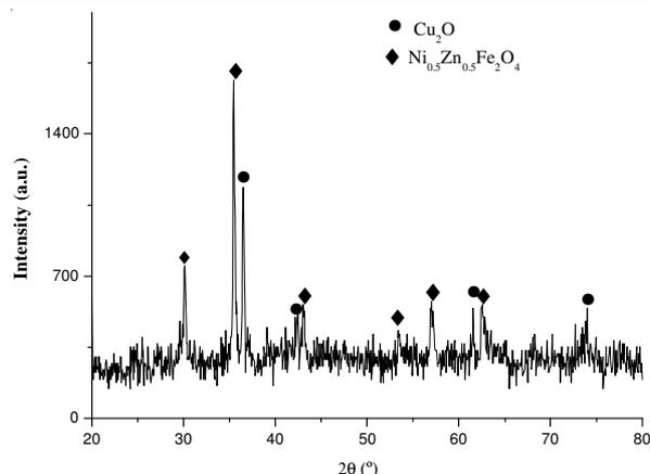
Fig. 3. XRD pattern of  $\text{Cu}_2\text{O}/\text{nickel-zinc ferrite composite microtubules}$
