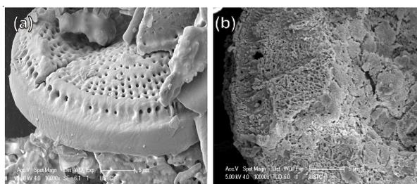
Fig. 1. SEM of raw diatomite (a) and lanthanum modified diatomite (b)
