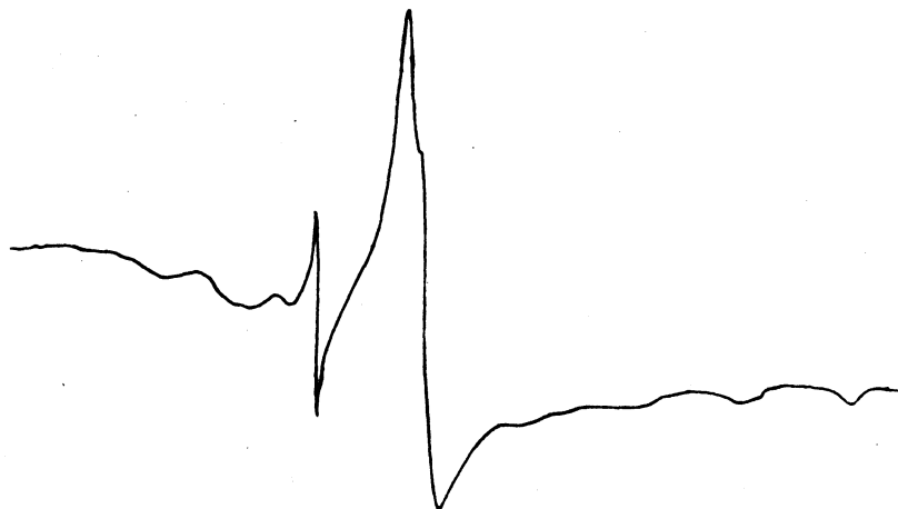
Fig. 5 ESR spectrum of Cu-phenoloxime in DMF at LNT
